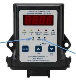
When setup as a grease spray system, this LED indicates the air solenoid status
