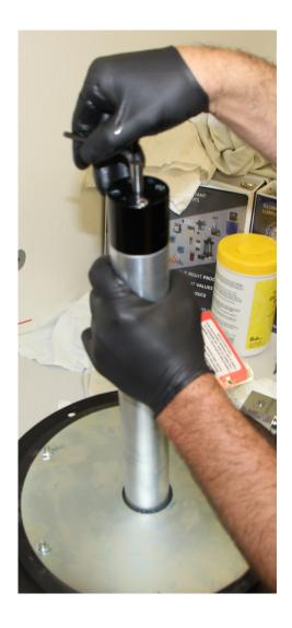
USING THE 3/16 ALLEN KEY, REMOVE THE TWO 1/4-28 X 2" SOCKET HEAD CAP SCREWS FROM THE BLACK PICK UP TUBE SPACER AND SET SPACER AND HARDWARE ASIDE.
