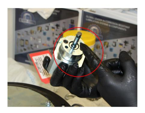
REMOVE PISTON FROM NEW INLET BLOCK, LUBE PISTON WITH CLEAN GREASE OR OIL FROM RESERVOIR, AND SLIDE PISTON INTO THE
