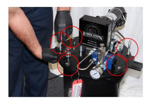
REMOVE THE SIX 3/8 BOLTS, NUTS, WASHERS, AND TWO EYE BOLTS FROM RESERVOIR LID. YOU WILL NEED TWO 9/16 END WRENCHES.
