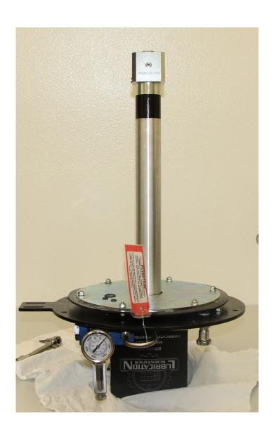
ONCE THE PUMP ASSEMBLY IS REMOVED FROM THE RESERVOIR, FLIP ASSEMBLY UPSIDE DOWN AND GENTLY LAY THE MOTOR SIDE ON SOMETHING SOFT OR ANYTHING TO PROTECT FROM COSMETIC DAMAGE.
