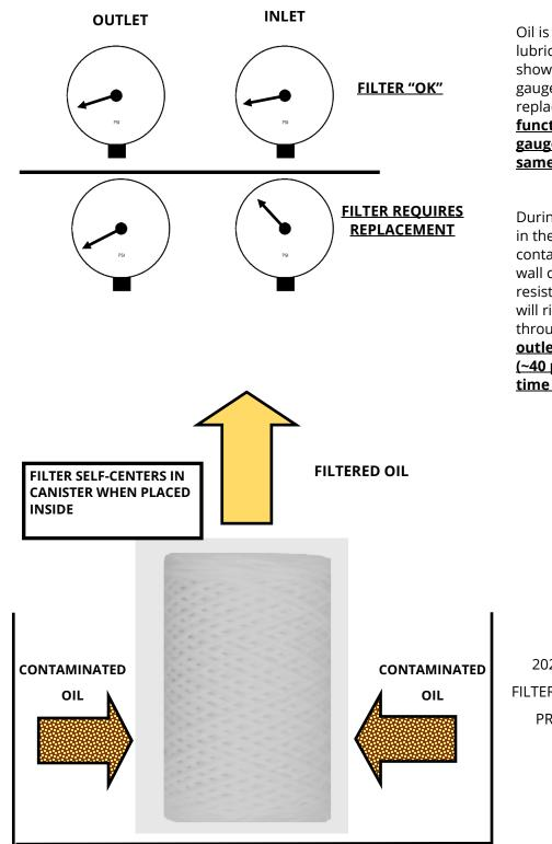
Oil is decontaminated by passing lubricant through the filter element as shown below. Installation of pressure gauges make indication of element replacement easy. <u>The filter is</u> <u>functioning properly when both</u> <u>gauges are at approximately the</u> <u>same psi level.</u>
