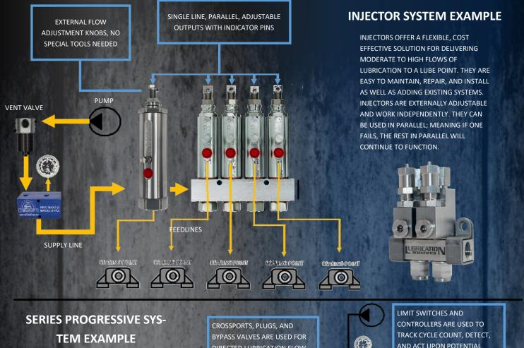
PRECISE LUBRICATION IS ESSENTIAL FOR PROPER MECHANICAL PERFORMANCE. PUMPS PROVIDE MEASURED PRESSURIZED LUBRICATION TO THE MASTER VALVE. THE MASTER VALVE DISTRIBUTES A MEASURED AMOUNT OF LUBRICATION TO ITS CORRE-SPONDING SECONDARY VALVES. SECONDARY VALVES DISTRIBUTE MEASURED LUBRICA-TION TO VARIOUS LUBE POINTS IN THE SYS-TEM.
